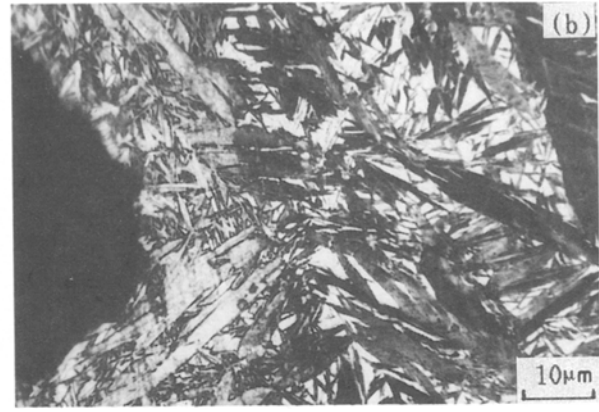
Figure 2 (a) Lower bainitic structure produced with insufficient isothermal transformation time. (b) Upper bainitic structure produced with insufficient isothermal transformation time.
